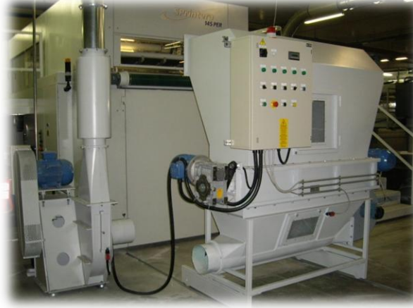
Ripping device and hopper on rails
